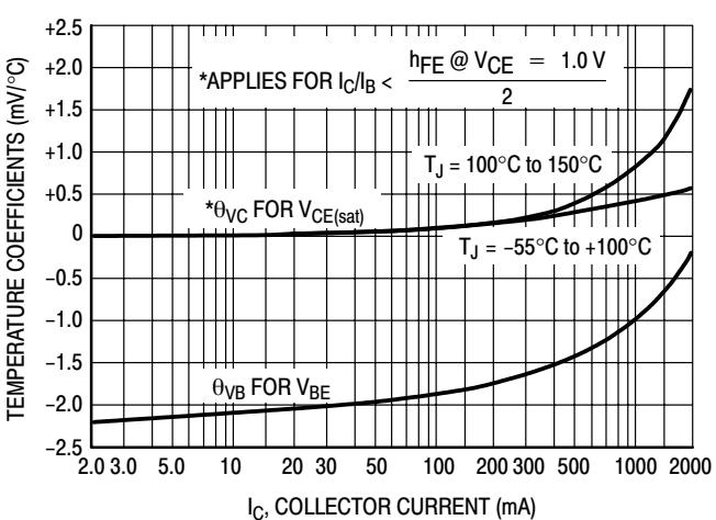
Figure 13. Temperature Coefficients
