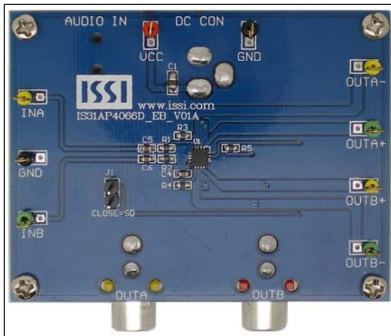
Figure 1: Photo of IS31AP4066D Evaluation Board
