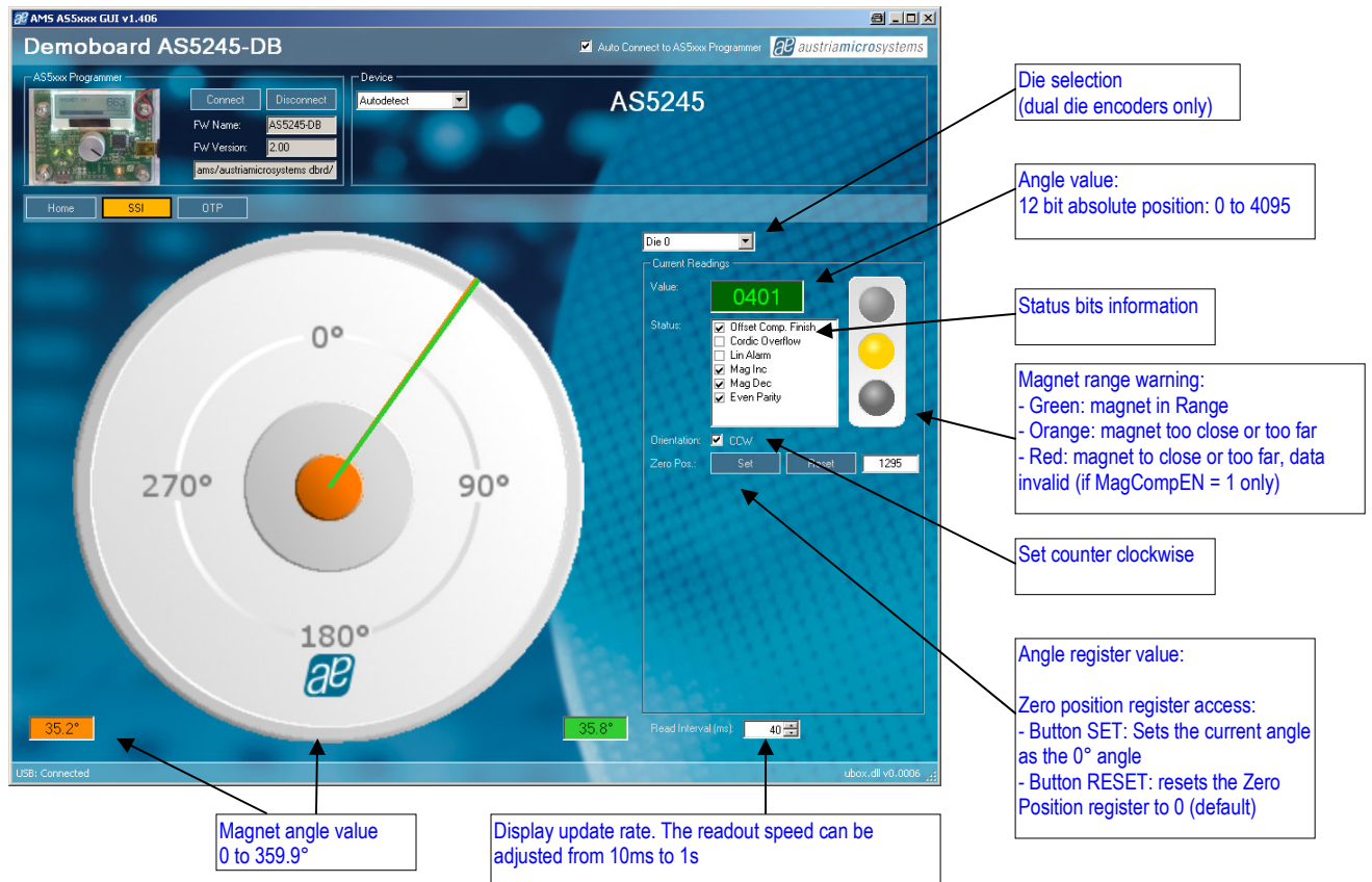
Figure 4: SSI tab, shows the SSI bus data of the selected encoder
