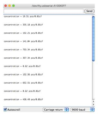
The result above consists of three parts: lowpulseoccupancy, ratio and concentration.
