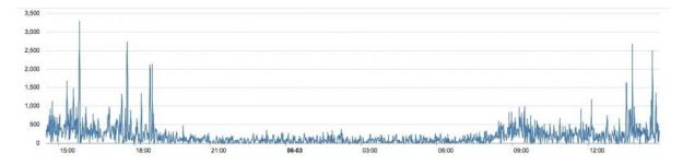
We can see the concentration of dust is very low in the evening, but it's higher in the afternoon. Maybe you can set a threshold value while the concentration is beyond a value. Also, if you wanna set the sensor more sensitive you can add a fan on the sensor, and add a 10k resistor between the Pin5 and Ground. More information please visit the blog of A.J.
