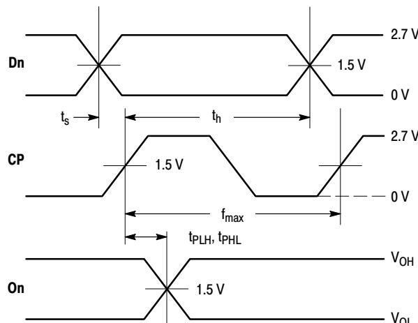
WAVEFORM 1 - PROPAGATION DELAYS, SETUP AND HOLD TIMES
