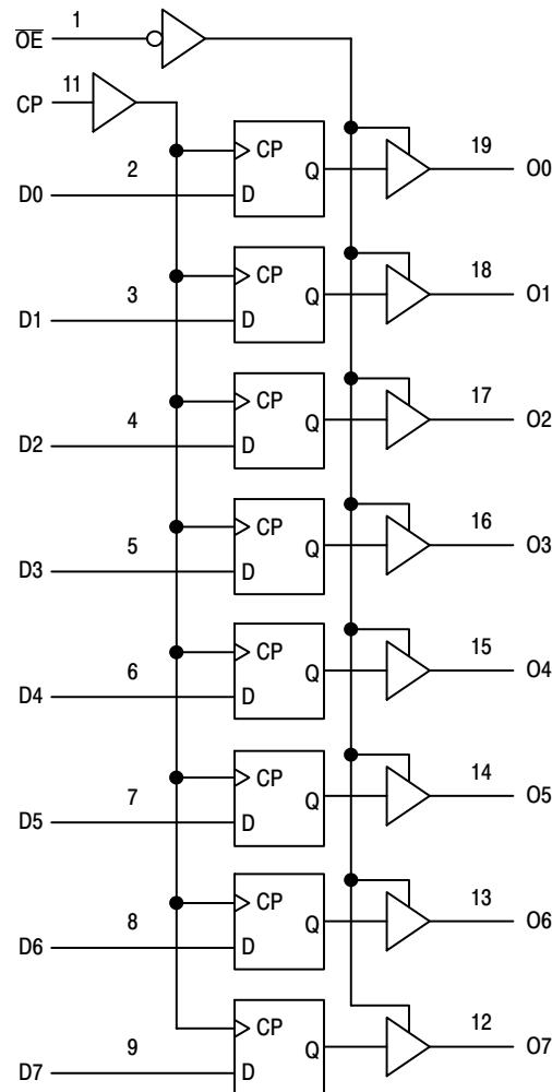
Figure 2. Logic Diagram
