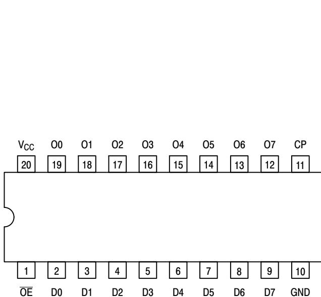
Figure 1. Pinout: 20-Lead (Top View)
