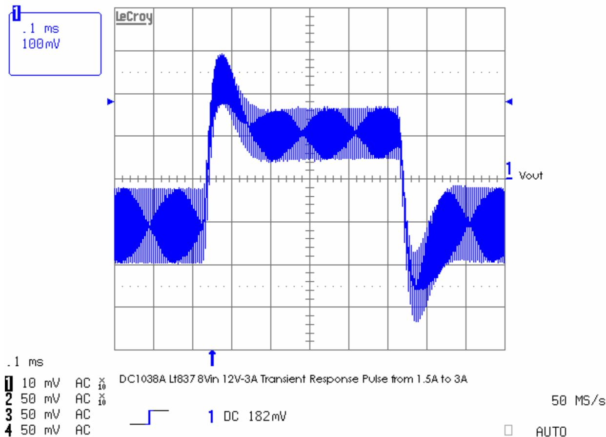
Figure 5. Transient Response Waveform at 18Vin and 1.5 - 3Aout
