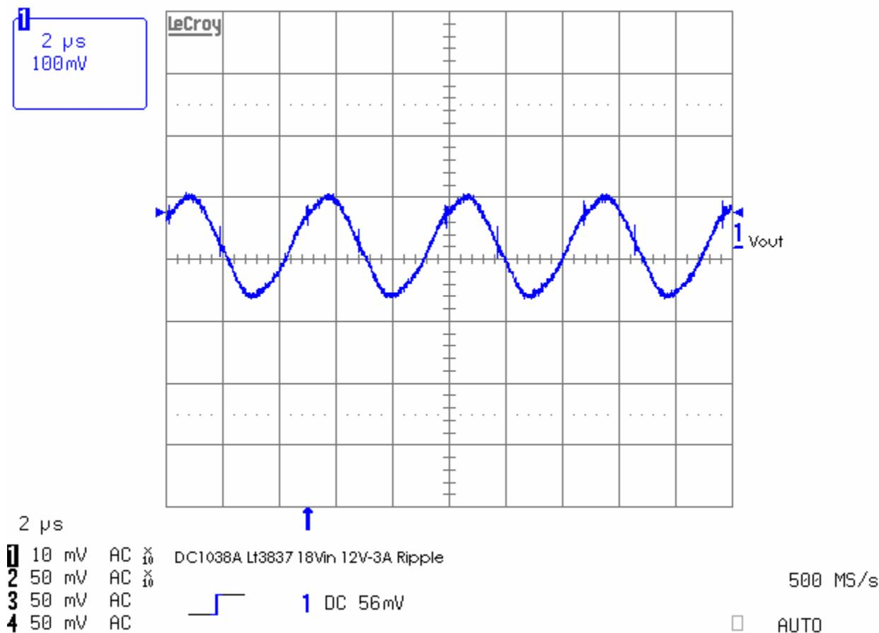
Figure 4. Output Ripple at 18Vin and 3Aout
