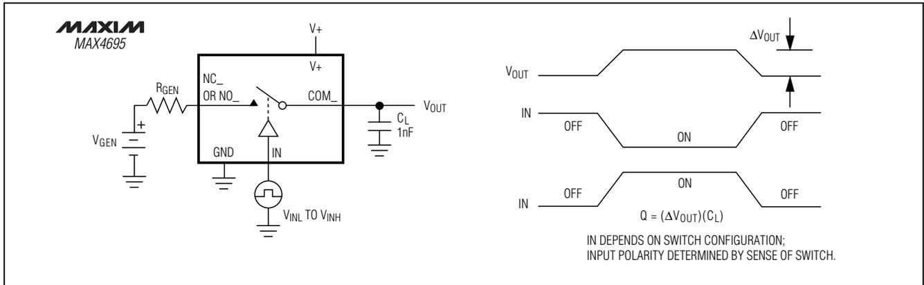
Figure 4. Charge Injection
