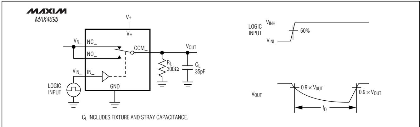
Figure 3. Break-Before-Make Interval
