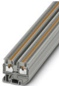
Mini feed-through terminal block, Connection method: Push-in connection, Cross section: 0.14 mm 2 - 1.5 mm 2 , AWG: 26 - 14, Width: 3.5 mm, Color: blue, Mounting type: NS 15
