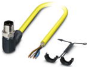
Sensor/Actuator cable, 4-position, PVC, yellow RAL 1021, shielded, Plug angled M12 SPEEDCON, A-coded, on free cable end, Cable length: 2 m
