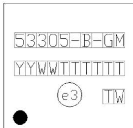
Figure 8.6. Si53305 Top Marking
