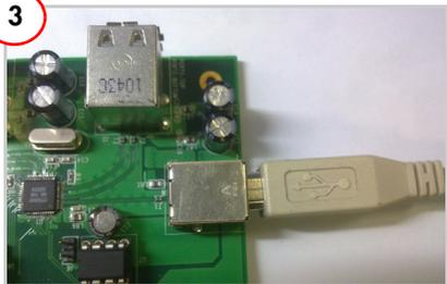
To connect to the PC, plug the USB A to B cable into the hub's upstream connector. Plug the other end of the cable into one of the PC's host controller ports.
