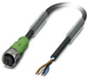
Sensor/actuator cable, 4-position, PUR halogen-free, black-gray RAL 7021, free cable end, on Socket straight M12 SPEEDCON, B-coded, cable length: 2 m
