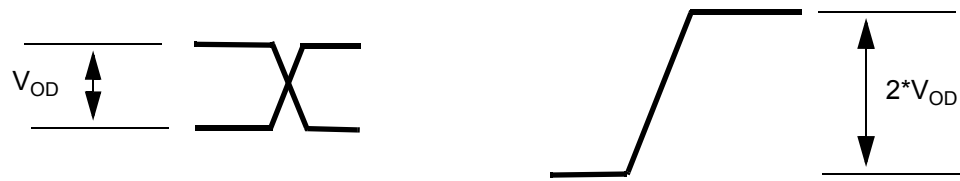
Figure 19 - Differential Output Voltage Parameter
