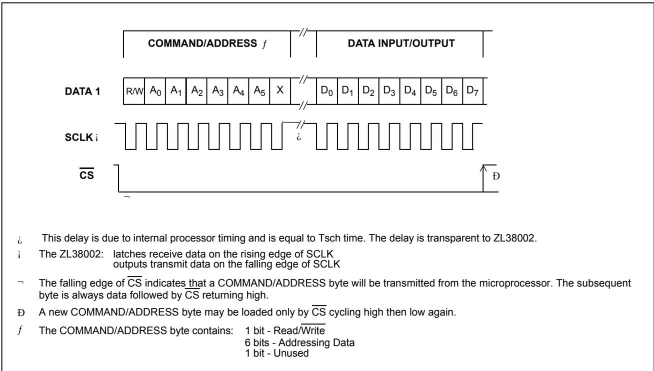
Figure 8 - Serial Microport Timing for Intel Mode 0
