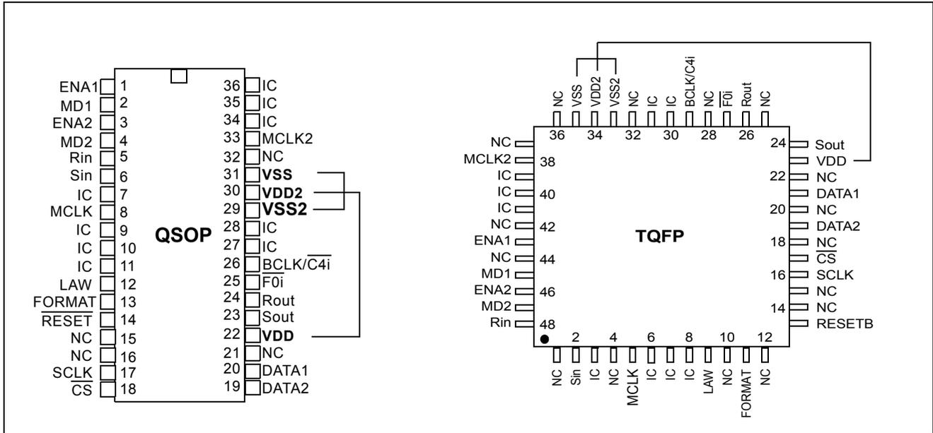
Figure 2 - Pin Connections
