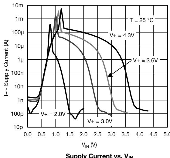
**Supply Current vs.  $V_{\text{IN}}$**
