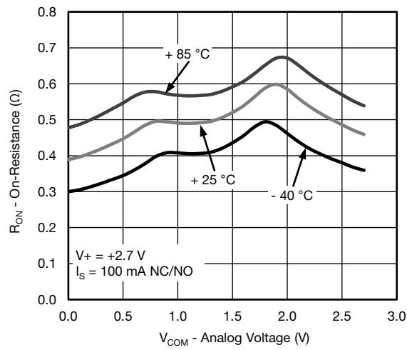
**$R_{\text{ON}}$  vs. Analog Voltage and Temperature**
