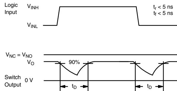
**Fig. 2 - Break-Before-Make Interval**
