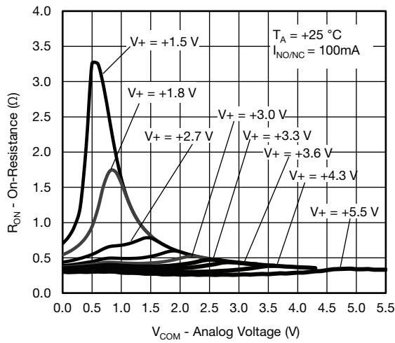
**$R_{\text{ON}}$  vs.  $V_{\text{COM}}$  and Supply Voltage**
