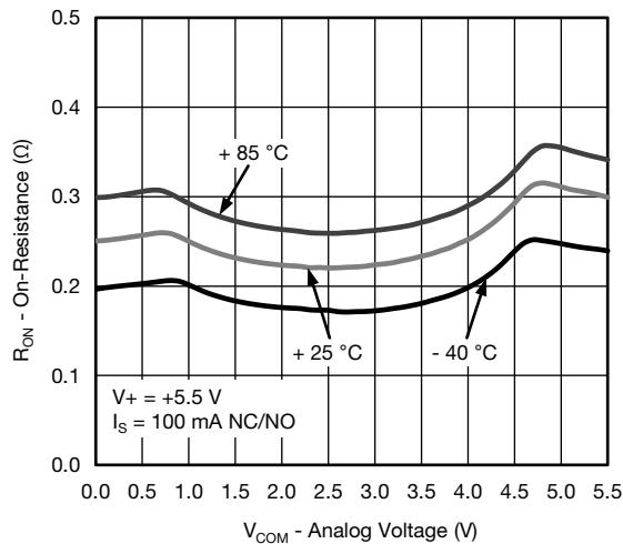
**$R_{\text{ON}}$  vs. Analog Voltage and Temperature**
