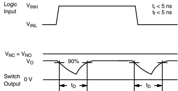
**Fig. 2 - Break-Before-Make Interval**
