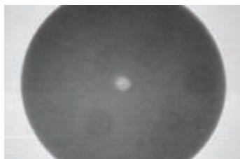
Ceramic Connector Cleaned with Novec Contact Cleaner
