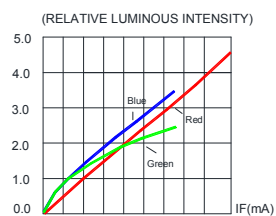
FIG.2 RELATIVE LUMINOUS INTENSITY VS. FORWARD CURRENT
