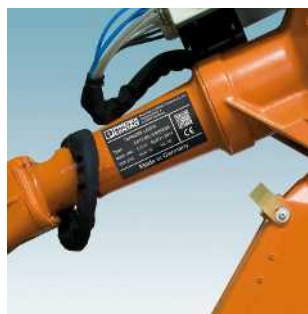
Laser device marking, laser foil
