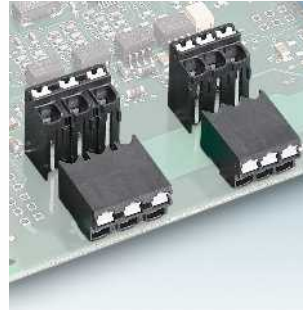
THR PCB terminal blocks with push-in spring connection up to 1.5 mm 2 , 3.5 and 3.81 mm pitch SPT-THR 1,5/ ...-H-3,5 P26 Page 10 SPT-THR 1,5/...-V-3,5 P26 Page 11
