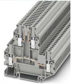
2.5 (4) mm 2 , 20 A, double-level terminal block with disconnect zone, test socket screw
