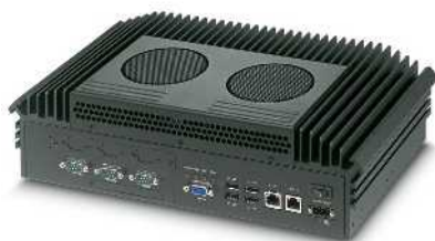
High-performance box PC for wall mounting
