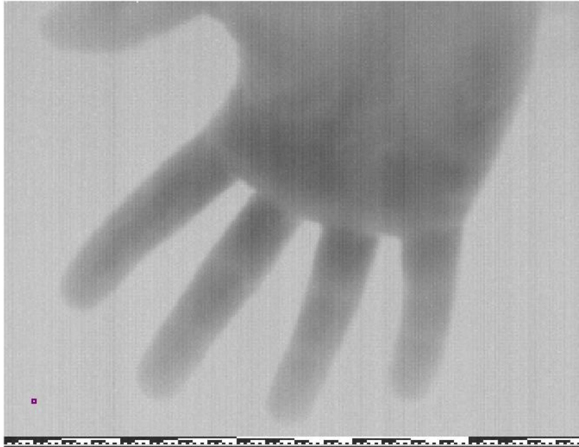
Figure 10: Raw tap A phase180 image of a hand with the test rows enabled
