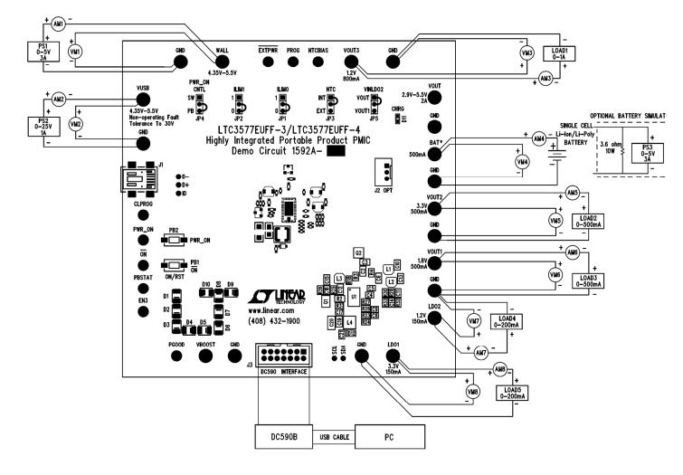
**Proper Measurement Equipment Setup**
