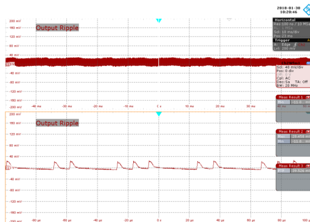
Figure 113 – 115 VAC 47 Hz, 25% Load. CH1: V_{OUT} , 40 mV / div., 10 ms / div. Zoom: 20 μs / div. Voltage Ripple ( V_{OUT(PK-PK)} ) = 39.5 mV).
