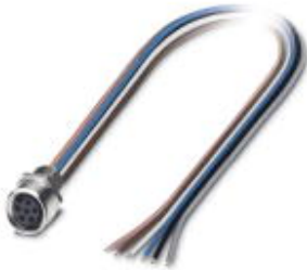
Sensor/actuator flush-type socket, 6-pos., M8, front/screw mounting with M8 fastening thread, with 0.5 m TPE litz wire, 6 x 0.14 mm²
