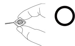
Don't pull fan with lead wires.
