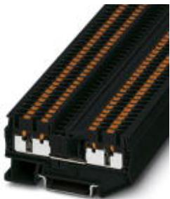
Feed-through terminal block, Connection method: Push-in connection, Cross section: 0.14 mm<sup>2</sup> - 4 mm<sup>2</sup>, AWG: 26 - 12, Width: 5.2 mm, Color: black, Mounting type: NS 35/7,5, NS 35/15
