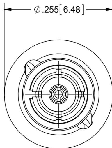
SMP INTERFACE PER MIL-STD 348 ACCEPTS  $\phi$  .015[0.38] PIN
