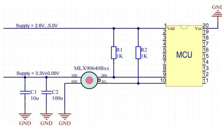
Figure 26 MLX90640 electrical connections
