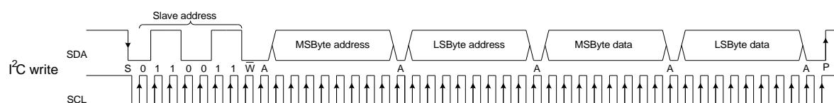
Figure 4 I<sup>2</sup>C write command format (default SA=0x33 is used)
