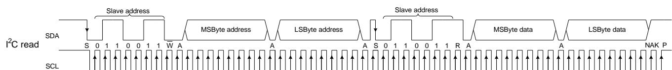
Figure 5 I<sup>2</sup>C read command format (default SA=0x33 is used)
