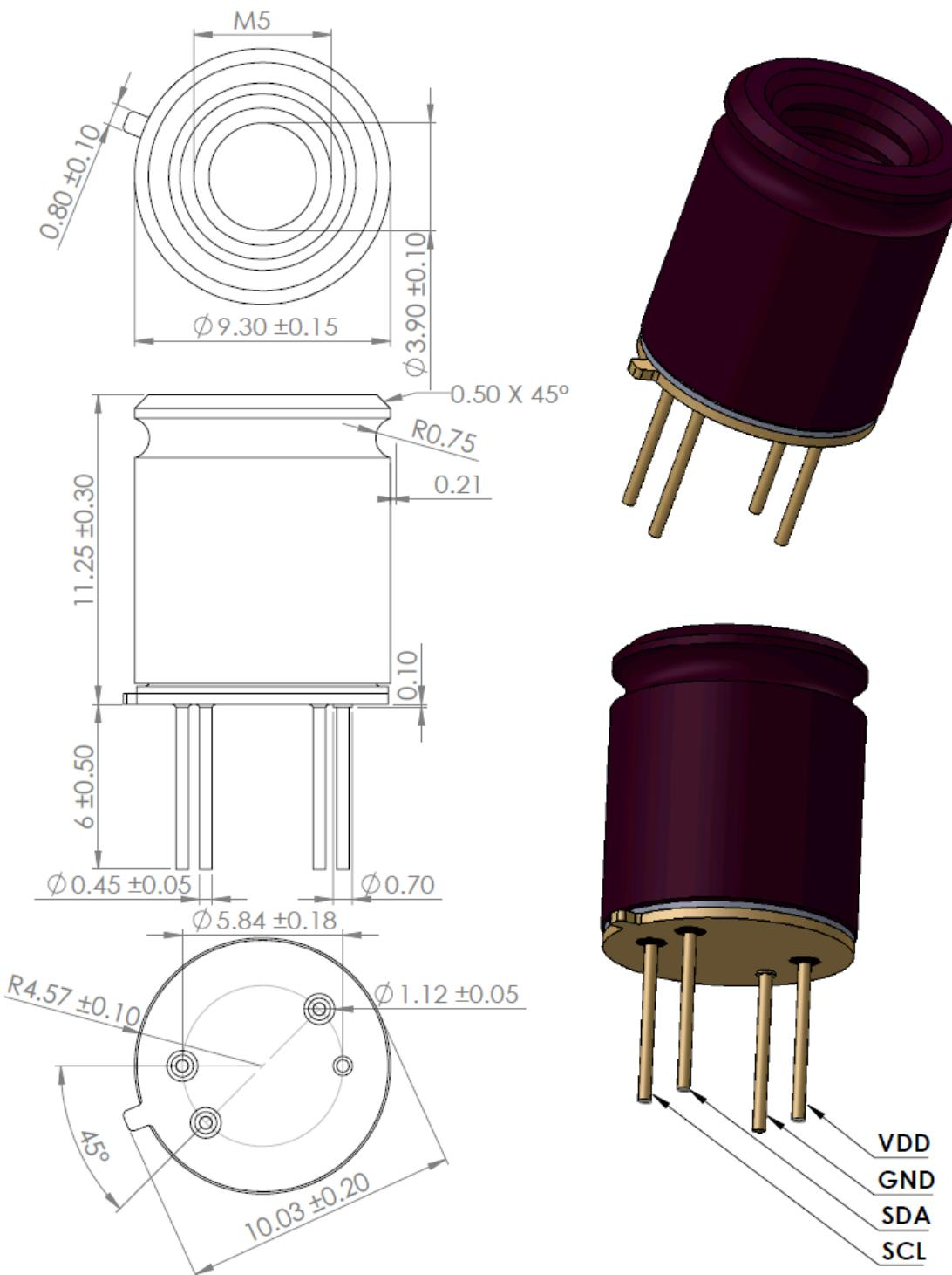
Figure 28 Mechanical drawing of 55° FOV device
