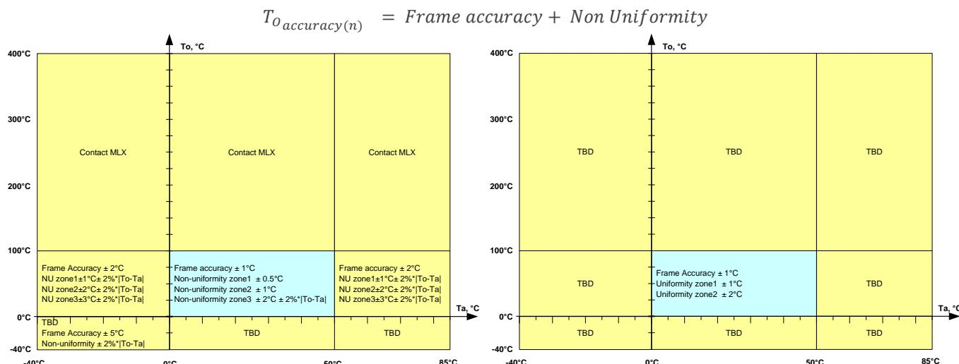
Figure 17 Absolute temperature accuracy – MLX90640BAA (left) and MLX90640BAB (right)
