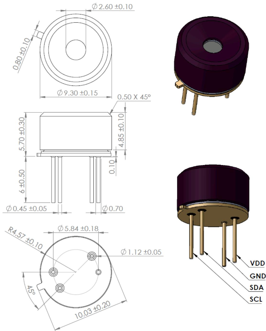
Figure 29 Mechanical drawing of 110° FOV device
