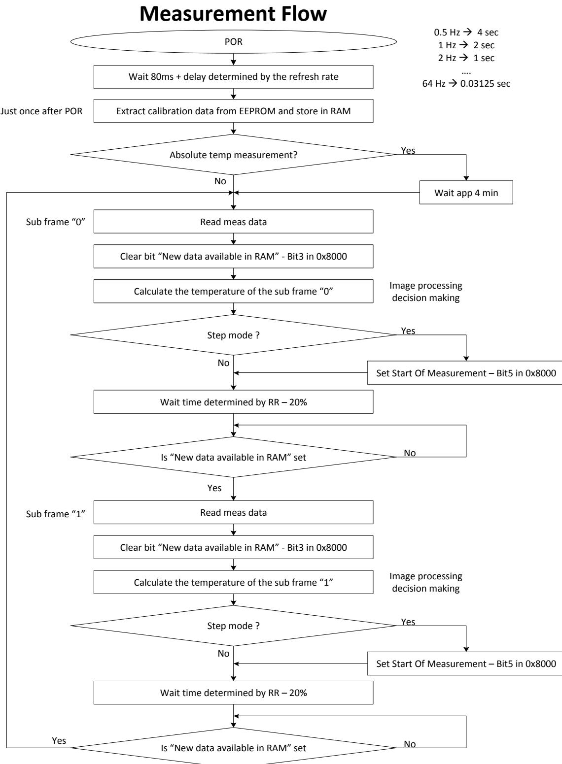
Figure 7 Recommended measurement flow
