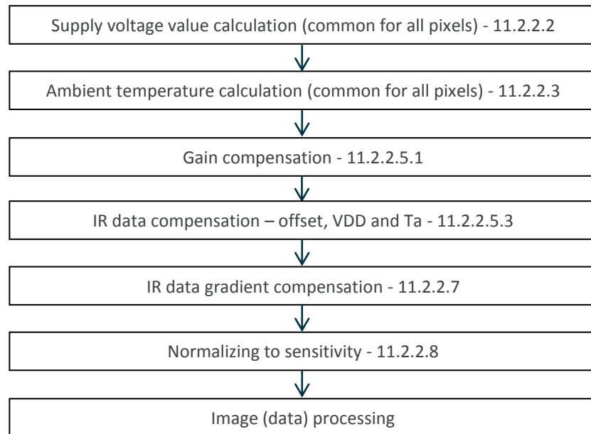
*Figure 27 Calculation flow in thermal image mode*
