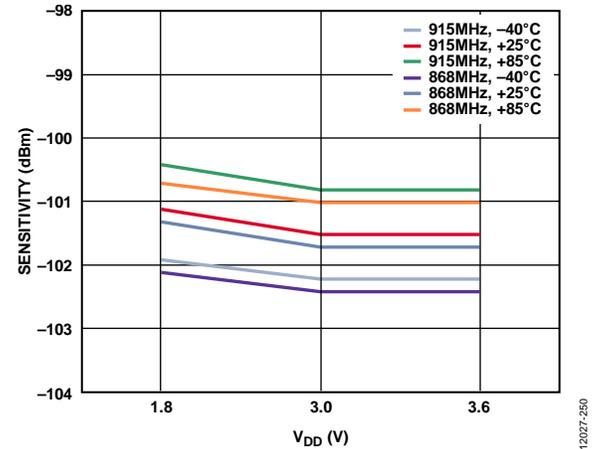
Figure 33. Receiver Sensitivity (Bit Error Rate at  $10^{-3}$ ) vs.  $V_{DD}$ , Temperature, and RF Frequency, Radio Profile F, FSK, (Minimum Recommended  $V_{DD} = 2.2\text{ V}$ , 1.8 V Operation Shown for Robustness)
