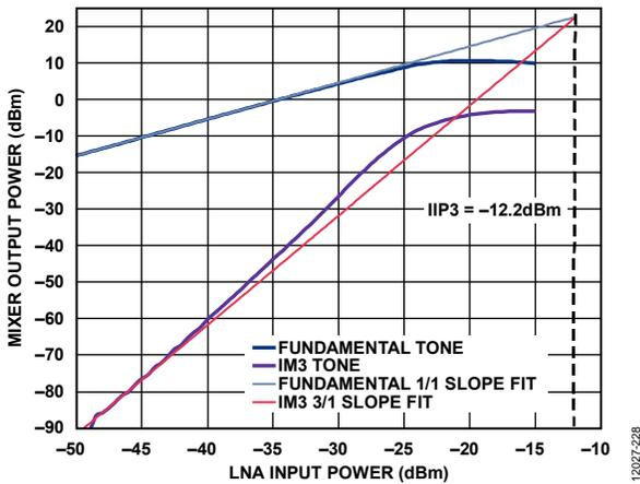
Figure 17. LNA/Mixer IIP3,  $V_{DD} = 3.0\text{ V}$ , Temperature = 25°C, RF = 915 MHz, LNA Gain = High, Mixer Gain = High, Source 1 Frequency = 915 MHz + 0.4 MHz, Source 2 Frequency = 915 MHz + 0.7 MHz
