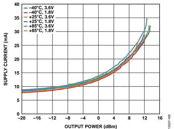
Figure 10. Supply Current vs. Output Power, Temperature, and V<sub>DD</sub> at 915 MHz (Minimum Recommended V<sub>DD</sub> = 2.2 V, 1.8 V Operation Shown for Robustness)
