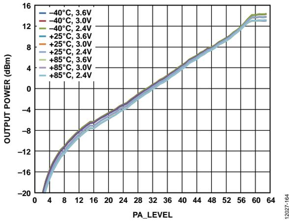
Figure 5. Output Power vs. PA\_LEVEL Setting, Temperature, and V<sub>DD</sub> at 433 MHz
