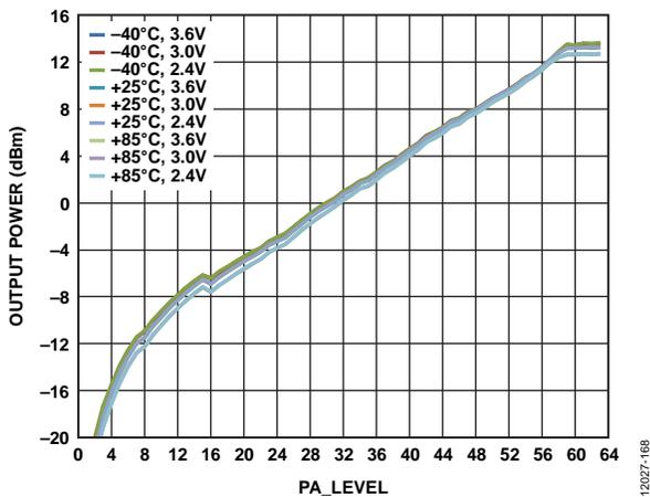
Figure 7. Output Power vs. PA\_LEVEL Setting, Temperature, and V<sub>DD</sub> at 915 MHz
