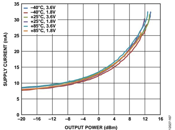
Figure 9. Supply Current vs. Output Power, Temperature, and V<sub>DD</sub> at 868 MHz (Minimum Recommended V<sub>DD</sub> = 2.2 V, 1.8 V Operation Shown for Robustness)
