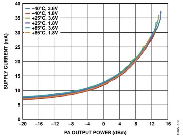
Figure 8. Supply Current vs. PA Output Power, Temperature, and V<sub>DD</sub> at 433 MHz (Minimum Recommended V<sub>DD</sub> = 2.2 V, 1.8 V Operation Shown for Robustness)
