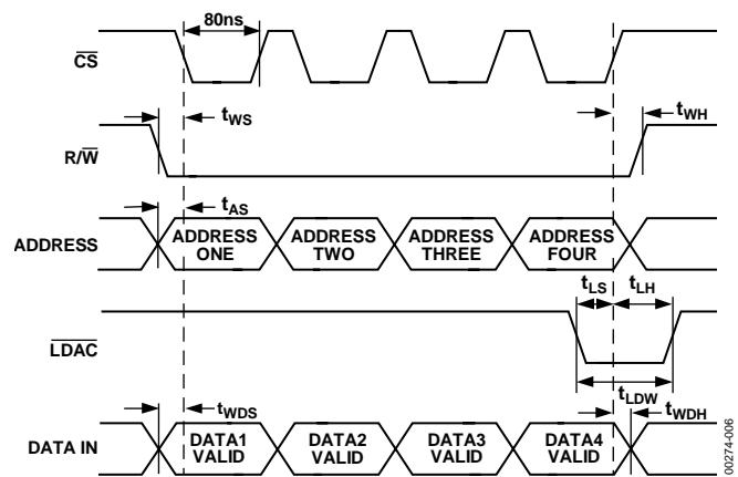
Figure 6. Double-Buffer Mode
