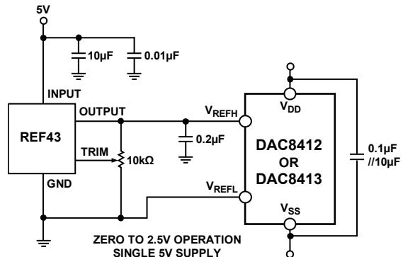
Figure 42.  $+5\ \text{V}$  Single-Supply Operation
