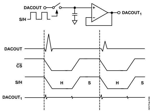
Figure 37. Data Output (Read Timing)
