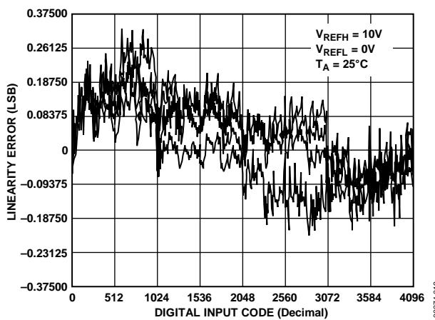
Figure 18. Channel-to-Channel Matching ( $V_{\text{SUPPLY}} = \pm 15\text{V}$ )
