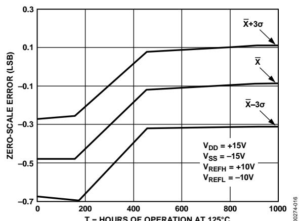
Figure 15. Zero-Scale Error vs. Time Accelerated by Burn-in
