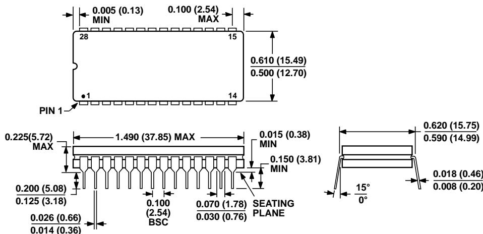
CONTROLLING DIMENSIONS ARE IN INCHES; MILLIMETER DIMENSIONS
