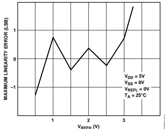
Figure 11. INL vs.  $V_{REFH}$
