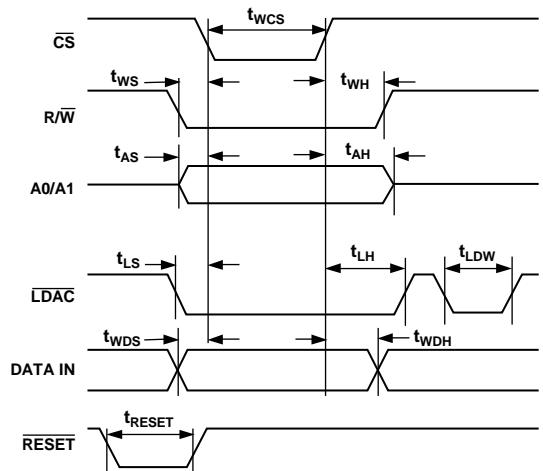
Figure 4. Data Write (Input and Output Registers) Timing
