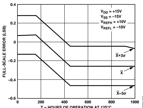
Figure 12. Full-Scale Error vs. Time Accelerated by Burn-in
