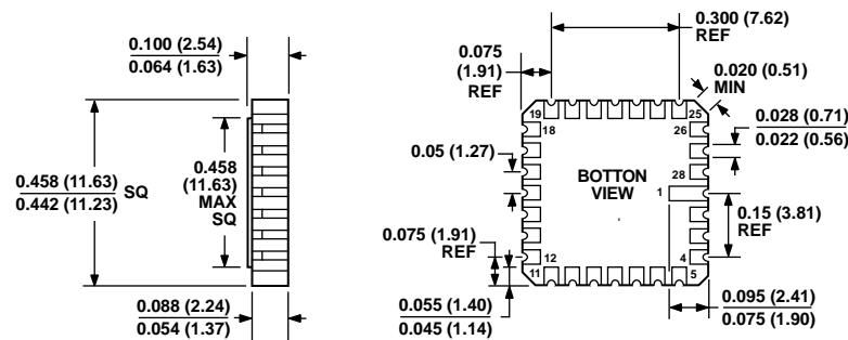
CONTROLLING DIMENSIONS ARE IN INCHES; MILLIMETER DIMENSIONS
