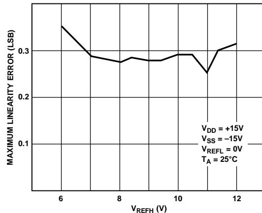
Figure 14. INL vs.  $V_{REFH}$
