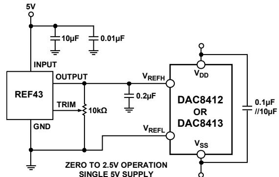
Figure 42.  $+5\ \text{V}$  Single-Supply Operation
