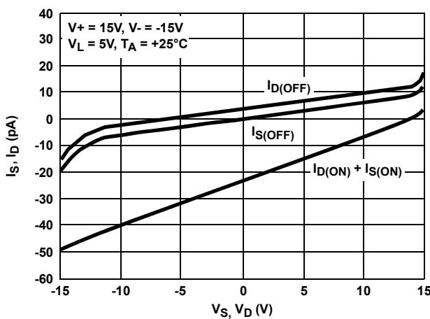
FIGURE 10. LEAKAGE CURRENTS vs ANALOG VOLTAGE
