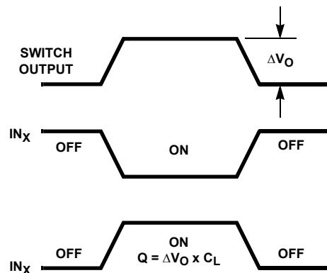
NOTE:  $IN_X$  dependent on switch configuration, input polarity determined by sense of switch.
