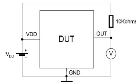
Note 1 -  $B_{OP}$  is determined by putting the device under magnetic field swept from  $B_{RPmin}$  up to  $B_{OPmax}$  until the output is switched on.
