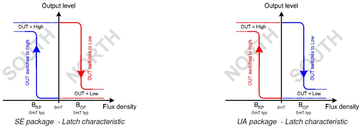
The device behaves as a latch with symmetric operating and release switching points ( $B_{OP}=|B_{RP}|$ ). This means magnetic fields with equivalent strength and opposite direction drive the output high and low.
