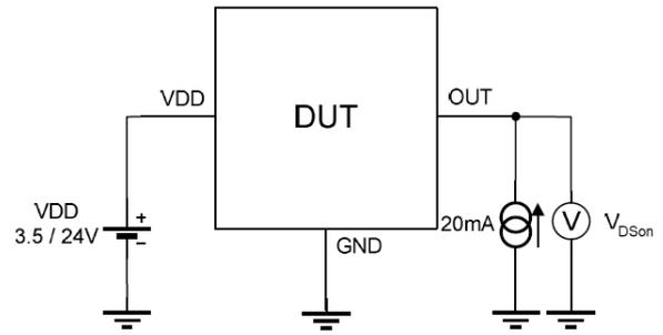
Note 1 - The output saturation voltage  $V_{DSon}$  is measured at  $V_{DD} = 3.5V$  and  $V_{DD} = 24V$ .
