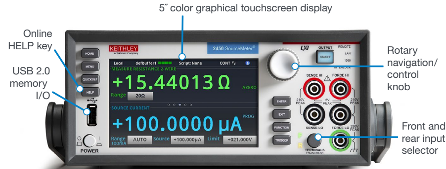
2450 front panel with high-resolution, capacitive touchscreen.
