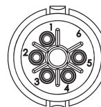
5 POSITION B-KEY #26 PIN & SOCKET CONTACT
