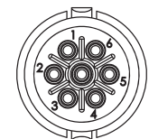
7 POSITION B-KEY #26 PIN & SOCKET CONTACT
