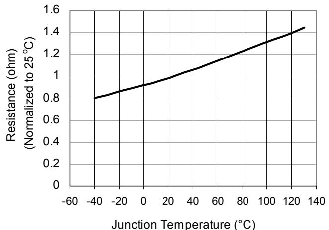
Figure 5. R<sub>ON</sub> vs. Temperature
