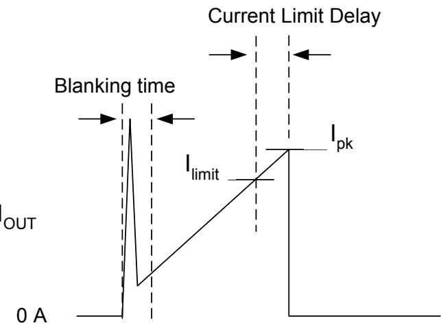
Figure 2. Graphical explanation of Current Limit terminology
