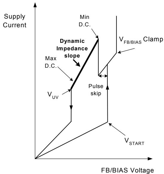
Figure 4. Supply Current vs. FB/BIAZ Voltage
