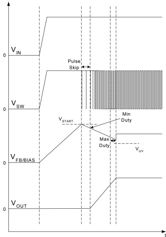
Figure 1. Power-up waveforms
