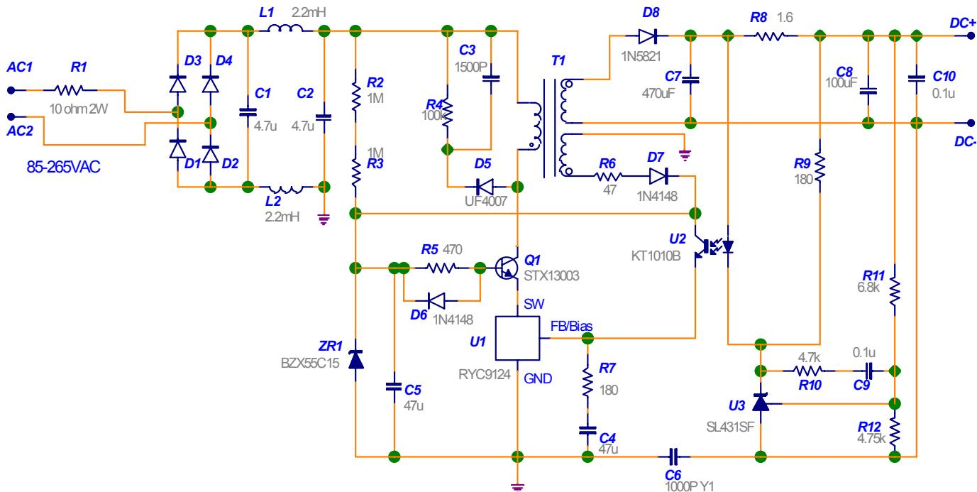
A typical application schematic is shown above, using the RYC91XX with a BJT as the high voltage transistor. The power supply operates over a universal input range (85–265 VAC) and delivers 6V, 700mA current which is adequate to charge most single-cell Lithium-ion batteries.
