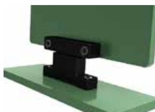
Right angle plug to straight receptacle
