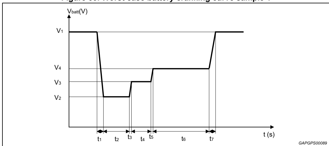
Figure 33. Worst case battery cranking curve sample 1
