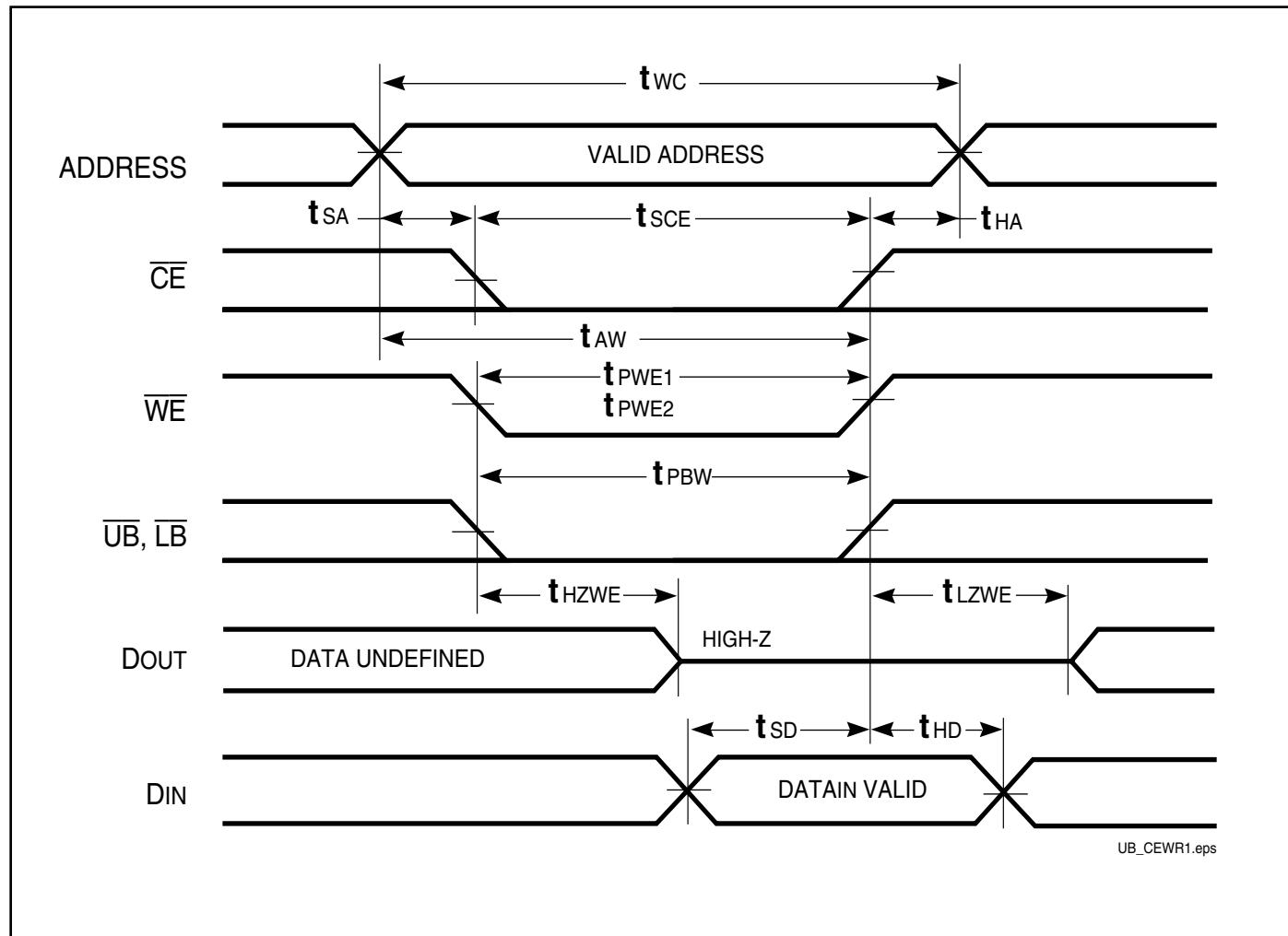
**WRITE CYCLE NO. 2<sup>(1)</sup> ( $\overline{WE}$  Controlled,  $\overline{OE} = \text{HIGH}$  during Write Cycle)**
