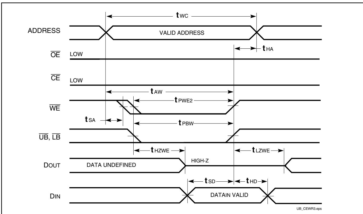
**WRITE CYCLE NO. 4 ( $\overline{\text{LB}}$ ,  $\overline{\text{UB}}$  Controlled, Back-to-Back Write) <sup>(1,3)</sup>**
