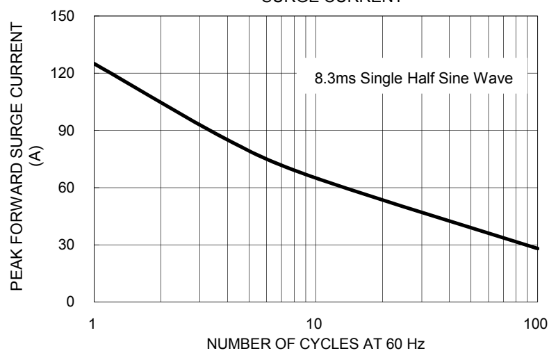
FIG. 3 MAXIMUM NON-REPETITIVE FORWARD SURGE CURRENT
