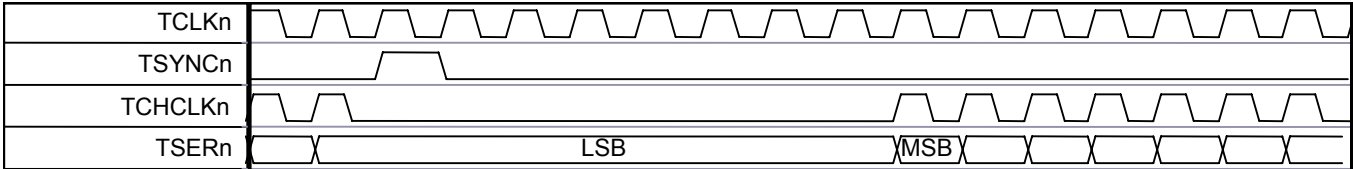
Figure 11-31. E1 Transmit-Side TCHCLKn Gapped Mode During Channel 1
