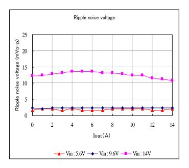
Fig. 12-3-6. Ripple Voltage v.s. Output Current
