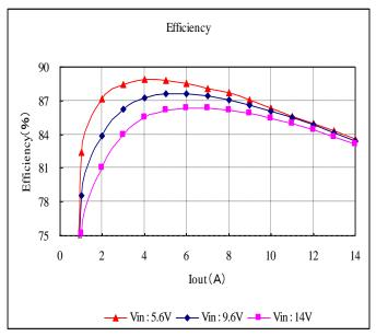
Fig. 12-3-11. Efficiency v.s. Output Current
