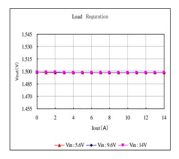
Fig. 12-3-10. Output Voltage v.s. Output Current
