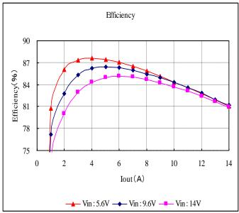
Fig. 12-3-14. Efficiency v.s. Output Current
