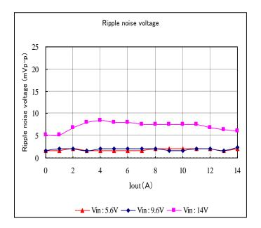
Fig. 12-3-12. Ripple Voltage v.s. Output Current
