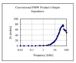
Fig. 12-2-2. Output Impedance of conventional product
