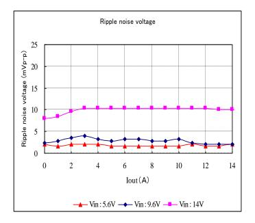
Fig. 12-3-15. Ripple Voltage v.s. Output Current
