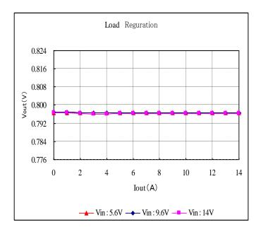
Fig. 12-3-16. Output Voltage v.s. Output Current
