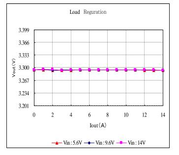
Fig. 12-3-1. Output Voltage v.s. Output Current
