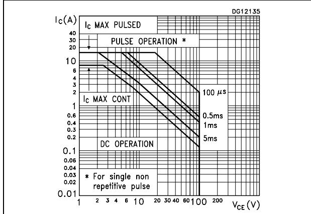
**Figure 3. Derating curve**
