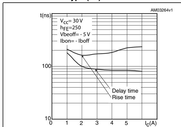
**Figure 13. Resistive load switching times for PNP type (on)**
