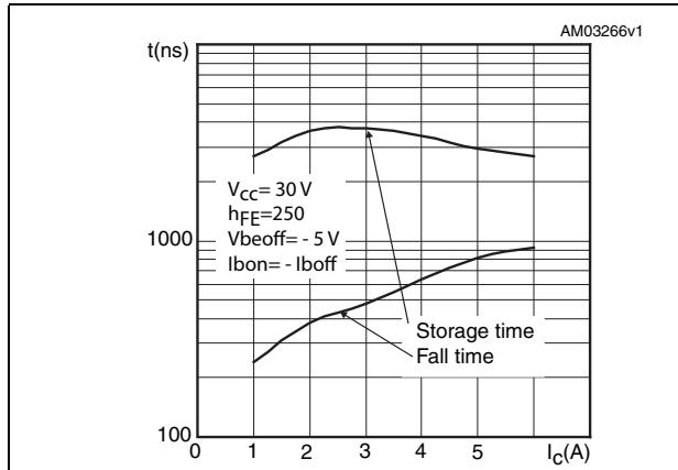
**Figure 15. Resistive load switching times for PNP type (off)**
