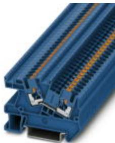
Installation terminal block, Push-in connection, Cross section: 0.14 mm<sup>2</sup> - 4 mm<sup>2</sup>, AWG: 26 - 12, Width: 5.2 mm, Color: blue, Mounting type: NS 35/7,5, NS 35/15
