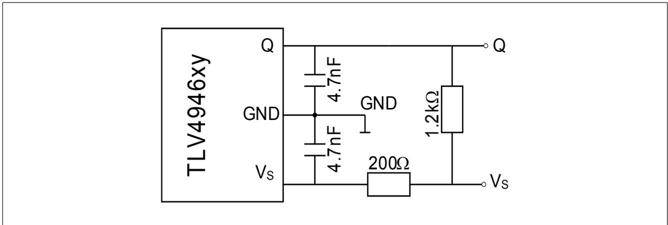
**Figure 5 Application circuit**
