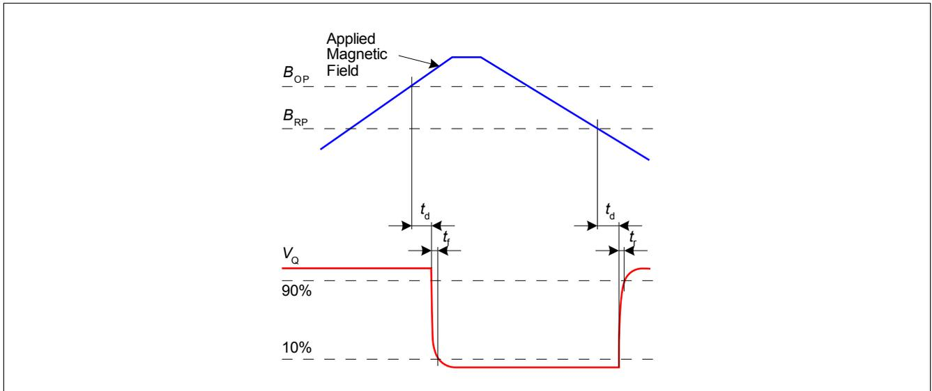
Figure 6 Timing Diagram
