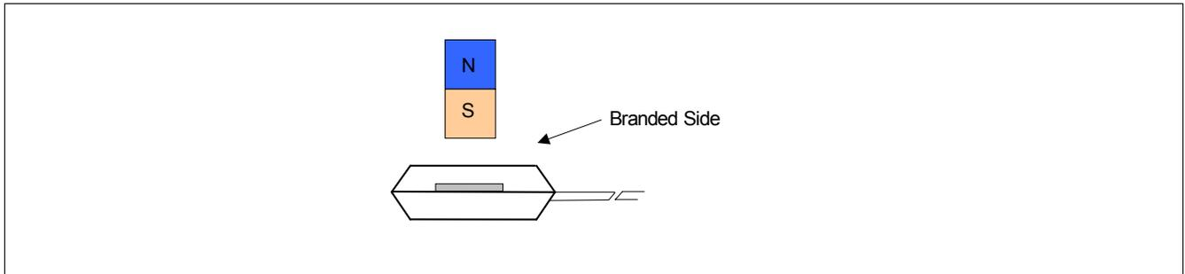
Figure 3 Definition of the Magnetic Field direction
